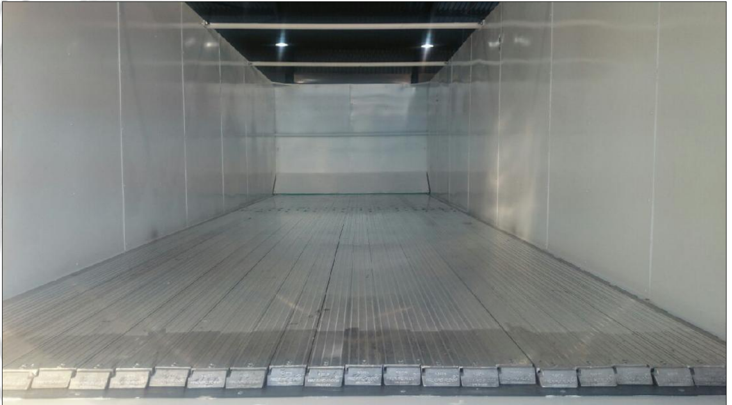
KEITH 21 plank aluminium walking floor in a rigid truck application.
