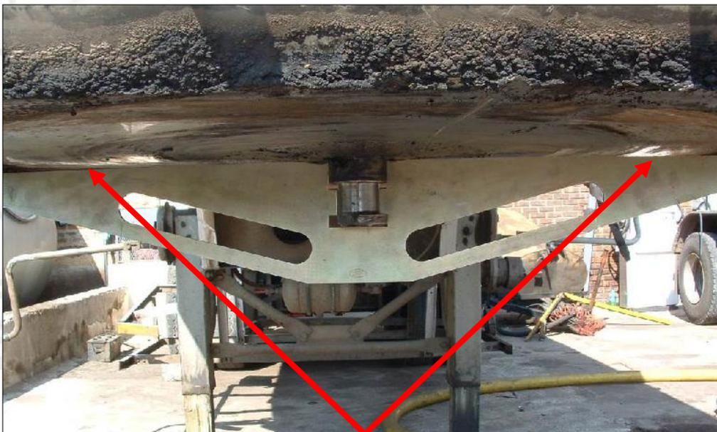
Max gap allowed new 1,5mm used 2mm. This skid plate will cause serious damage to any fifth wheel
