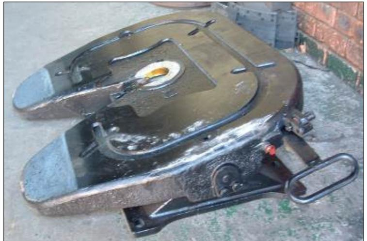
The following question is: where would you find spares for this fifth wheel, and how do you maintain it? On closer inspection it was found that Jost spares do not fit in the locking mechanism of this untraceable fifth wheel.
