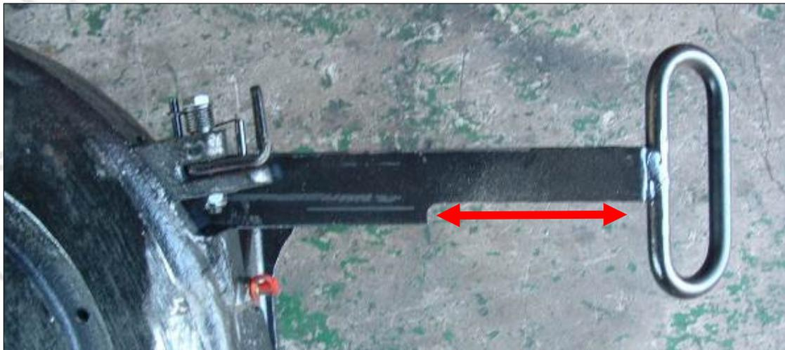
This handle has no wear indicator; even though it does have an adjusting bolt there is no way of knowing when the locking mechanism components (if obtainable) need to be replaced. Should this fifth wheel have been legal, this would unnecessarily complicate maintenance requirements.
