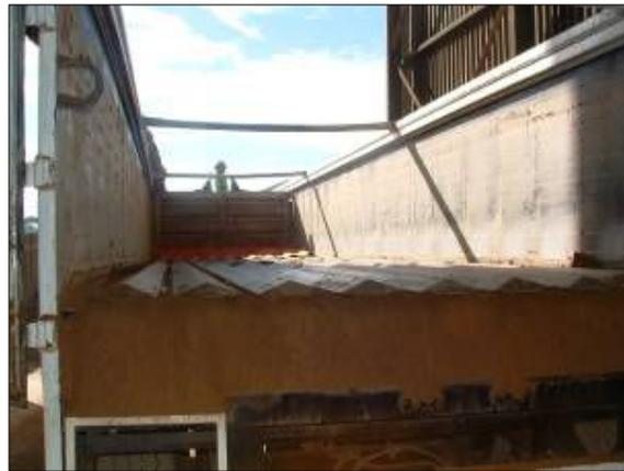
The driver is pulling the tarp back into position for the next load. Note how clean the floor has been swept while offloading.
