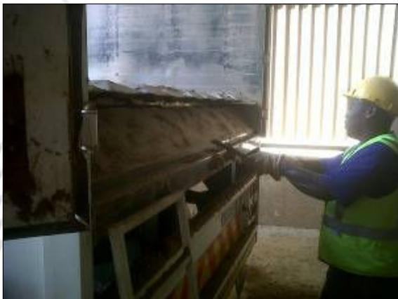
The driver is scraping the last bits of product from the end of the domex floor planks. Close the doors, the floor is now ready for the next load.
