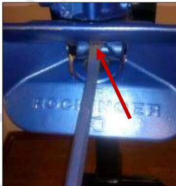
8. Bottom guide bush, min inner diameter 35,9mm
