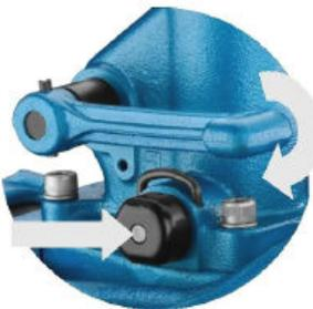
The **Jost-50** features a safety pin complete with locking indicator, and a rotating locking pin for even wear to prolong service life, and our standard **Jost** automotive e-coat paint to prevent corrosion. The large rubber cushions of the **Jost-50** tow hitch also reduces shock loading minimising wear and associated damage to the drivetrain of the towing vehicle.
