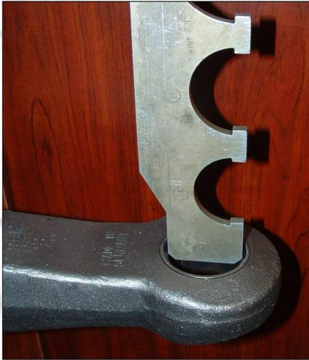
Measuring the 40 and 50mm towing eye has always been difficult. They eye wears in the centre where it is making contact with the tow hitch's outer ball edge of the pin. Using the traditional **J909L Jost No-Go Gauge** as prescribed, has always left more questions than answers. The area that the tool needs to enter is not affected by wear, thus the **J909L No-Go Gauge** cannot reach the area it is supposed to measure.
