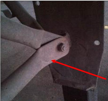
Ensure that the legs are parallel and aligned, they should be installed at 90 degree angles in relation to the chassis over the length and width of the chassis. Bracing on the leg should be minimum 45 degrees at all times. Also check the mounting bracket for deformation and cracks. Damaged bracing as shown here should be removed and repaired immediately.
