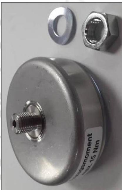
The JOST hubodometer needs to be fitted on the right hand side of the vehicle on the centre most axle of the axle group. The hubodometer has to be fitted dead center; oscillations caused by an un-balanced fitment will impair service life and the accuracy of the unit.
