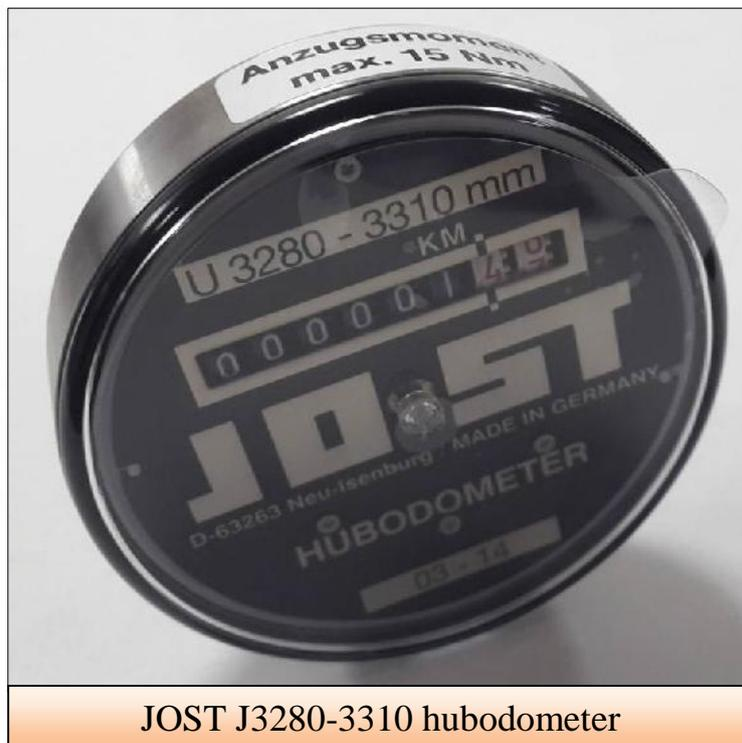
Trailers do not have odometers and do not necessarily stay hitched to one particular truck tractor, how many kilometers has your trailer done, and are you servicing the trailer at adequate intervals? The JOST hubodometer is an inexpensive solution to determine kilometers covered by the trailer from date of fitment.
