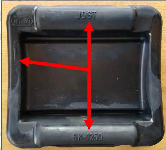
**JOST** name, part number and direction for installation arrow clearly visible, this is **JOST SK-1259 2" rubber**.
