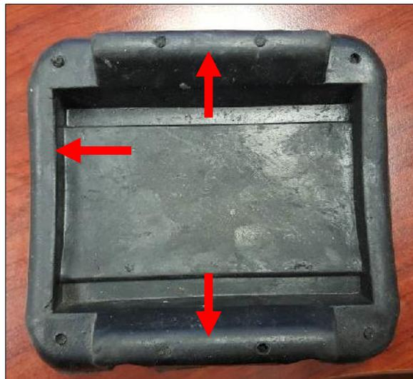
This is **not JOST**, no traceability, no name, no part number, no date of manufacture, no installation direction arrow, this rubber tested 3 times softer than a **JOST** original rubber.
