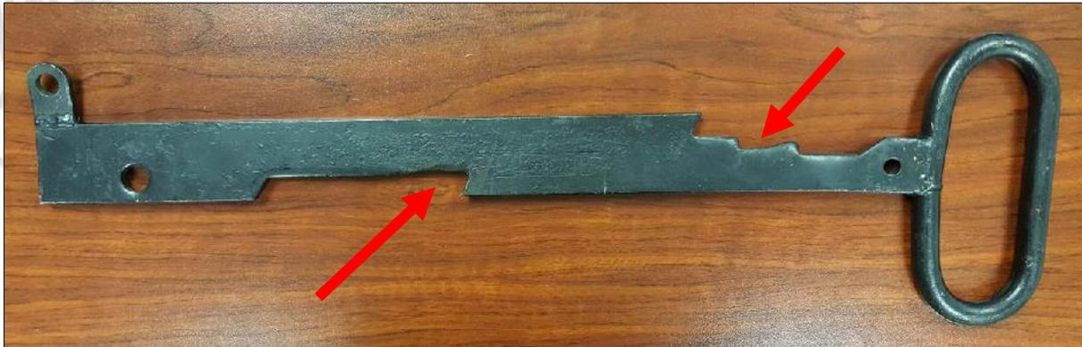
What not to do: This is a **JOST JSK37C** handle that has been remanufactured to fit a **JOST JSK36C** fifth wheel. Please do not change or remanufacture any critical safety components!
