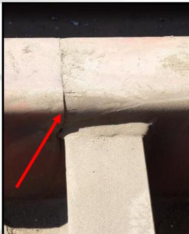
Cracked skid plate support structure too light to support the load of the trailer
