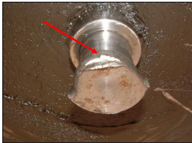
Cheap un-known kingpin flange broke away causing the trailer to fall and thousands of Rands in damages
