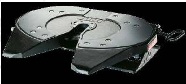
These plastic liners do not require greasing, only a thin layer of oil which is spread over the Teflon liners to prevent the semi-trailer rubbing plate from “biting” into the liners and to facilitate ease of steering. This results in a much cleaner operation.
