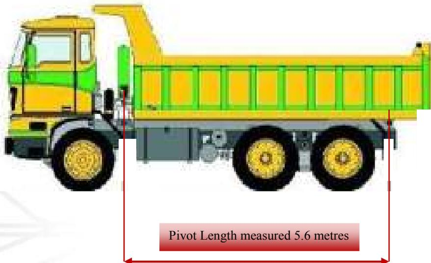
The tipping angle is determined by the customer or body builder depending on the length of the bucket and the load to be tipped.
